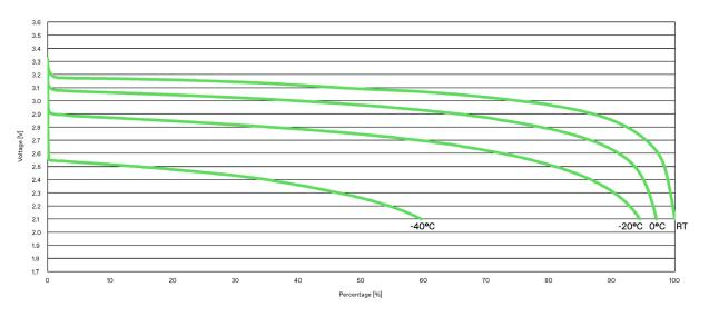
The diagram shows the latest measurement results for the discharge capacity of the HPB Solid-State Battery at room temperature (RT), 0 °C, -20 °C and -40 °C. It clearly shows that even at -20 °C the battery still has well over 90 % of the usable capacity that it has at room temperature.
