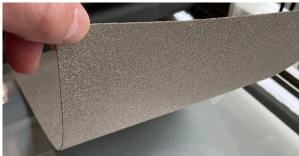
Open-pore nickel foam with a 3D structure
